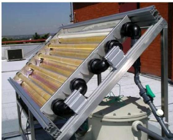
**Figure 1.6** Solar photoreactor for water disinfection test with the photosensitizing material into the glass tubes of the CPC. (Adapted from reference 101)
