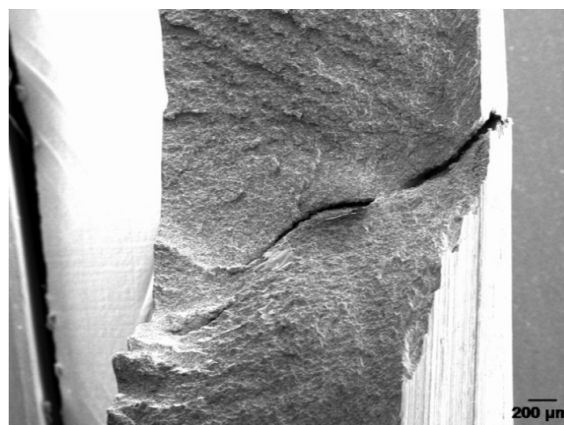
Figure 5.20 SEM image showing a full view of fracture surface covering complete thickness of the sleeve.
