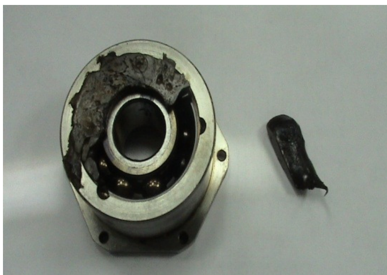
Figure 4.22 Bearing polyamide cage material damage during hot test at 315°C
