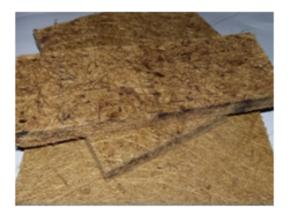
Figure 3.2: Medium density fibre boards manufactured from coir
