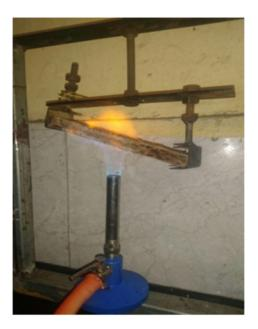
Figure 6.9: Resistance to flame spread test apparatus
