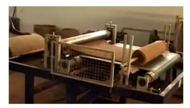
Figure 3.5: Glue Spreading Machine
