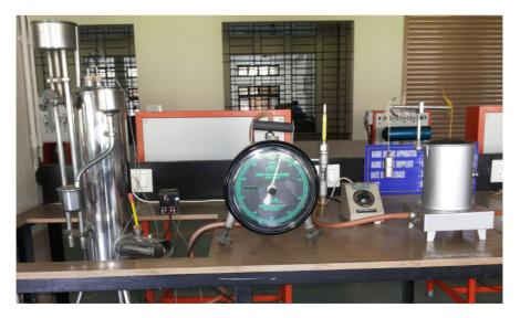
Figure 6.2: Junkers gas calorimeter apparatus
