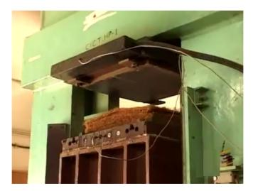
Figure 3.6: Hydraulic Hot Press
