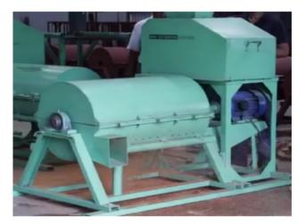
Figure 3.3: Mobile Fibre Extraction Machine
