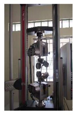
Figure 5.2: Universal Testing Machine for measuring tensile, bending and compressive properties of coir fibre boards
