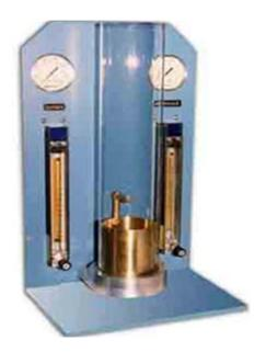
Figure 6.1: Limiting Oxygen Index Tester
