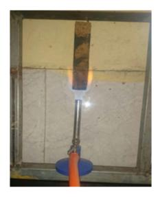
Figure 6.8: Rate of burning test apparatus
