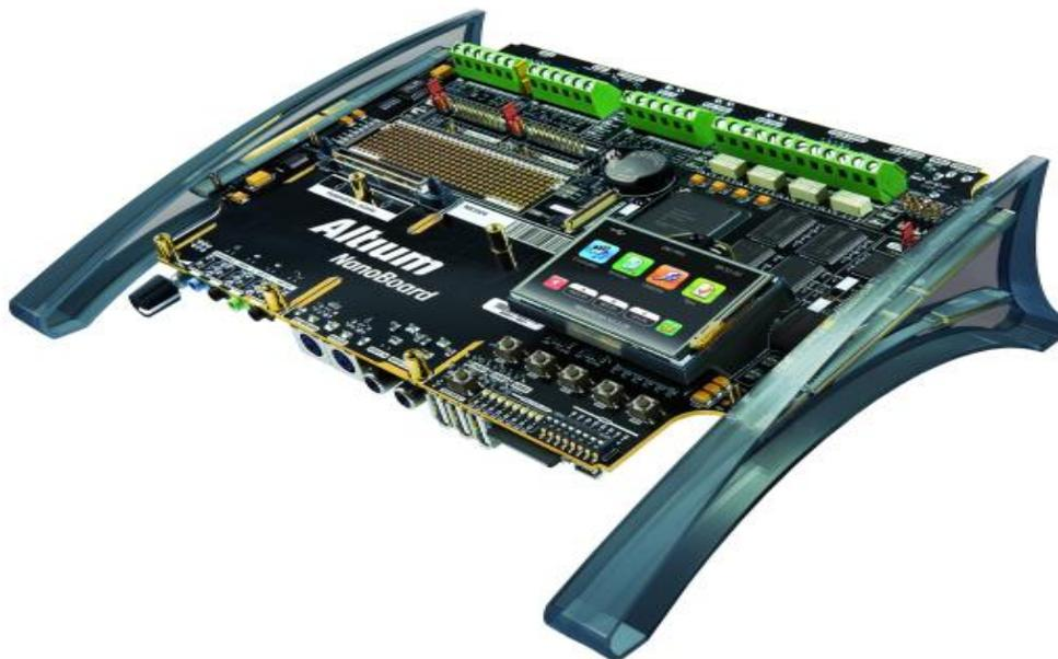
Fig 1.7 Altium NB3000 NanoBoard
