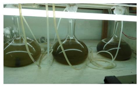
Fig. 4.7 Inoculum preparation for upscale cultivation of *Navicula phyllepta* in 3L Haffkine flask under laboratory conditions
