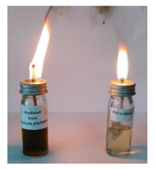
Fig. 3.7 Flame of biodiesel and petro-diesel
