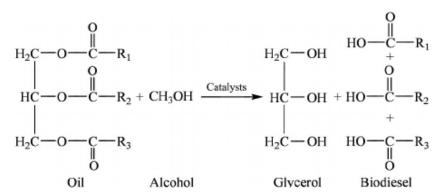
**Fig. 1.2** Transesterification reaction of microalgal lipids resulting in biodiesel and byproduct of glycerin (Ahmed et al., 2015)
