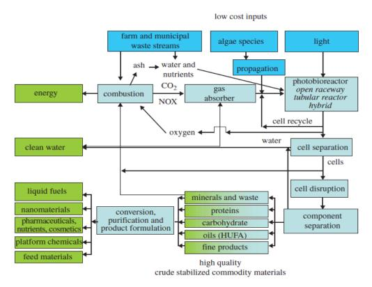
Fig. 1.5 Marine algal bio-refinery (Greenwell et al., 2009)
