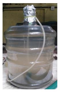
Fig. 4.10 Auto settling cells of diatom N. phyllepta by stopping aeration
