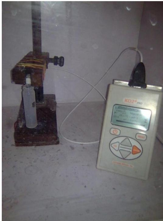
**Fig. 2** Optical photograph of a KD2 Pro thermal conductivity meter in which a platinum hot wire is immersed in the nanofluid which acts as both the heater and temperature sensor.
