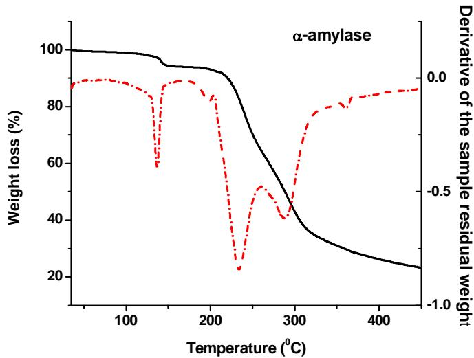
**Figure: 3.2** Thermogram of  $\alpha$ -amylase
