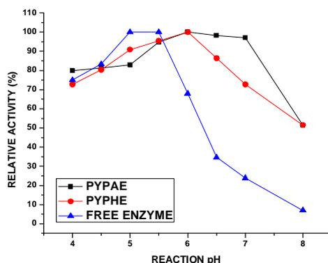
**Figure: 3.58:** Effect of pH on the relative activity of free and immobilized enzymes on copolymers
