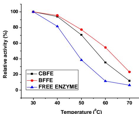
**Figure: 4.34:** Thermal stability of free and immobilized  $\alpha$ -amylase
