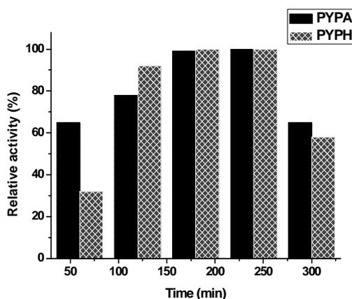
**Figure: 3.54:** Effect of contact time on immobilized enzyme relative activity
