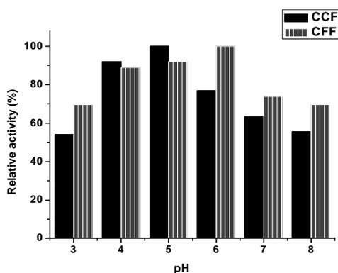
**Figure: 4.8** Effect of immobilization pH on the relative activity of  $\alpha$ -amylase
