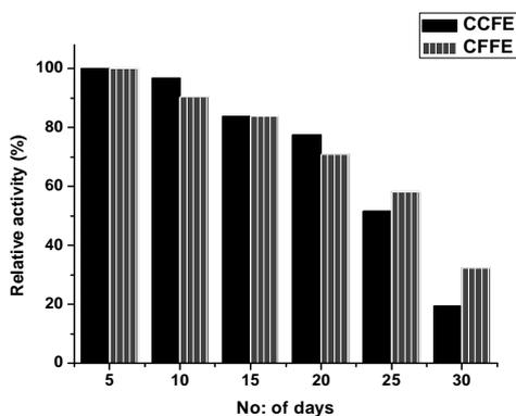
**Figure: 4.18:** Storage stability studies for immobilized enzymes on treated and functionalized coconut fibers
