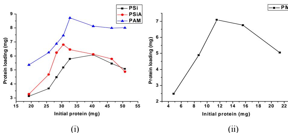
**Figure: 3.70** Influence of initial protein concentration on protein loading on to supports (i) PSi, PSiA, PAM (ii) PM
