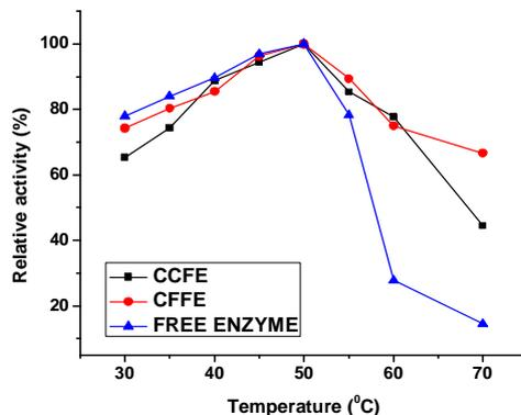
**Figure: 4.14:** Effect of temperature on relative activity of free and immobilized  $\alpha$ -amylase.
