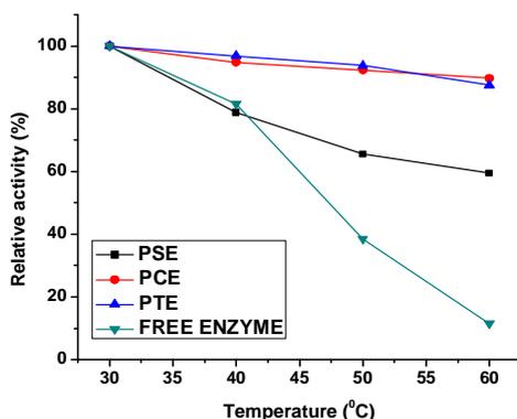
**Figure: 3.28:** Thermal stability of free and immobilized  $\alpha$ -amylase
