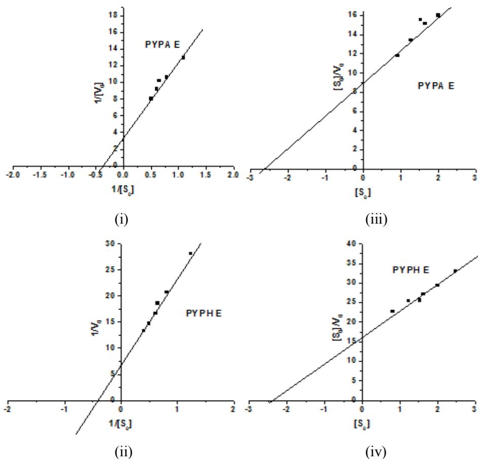
**Figure: 3.62:** Lineweaver-Burk plots for  $\alpha$ -amylase immobilized on copolymers (i) PYPA (ii) PYPH. Hanes-Woolf plots (i) PYPA (ii) PYPH
