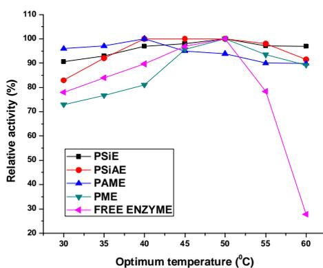
**Figure: 3.74:** Effect of temperature on the relative activity of free and immobilized enzyme
