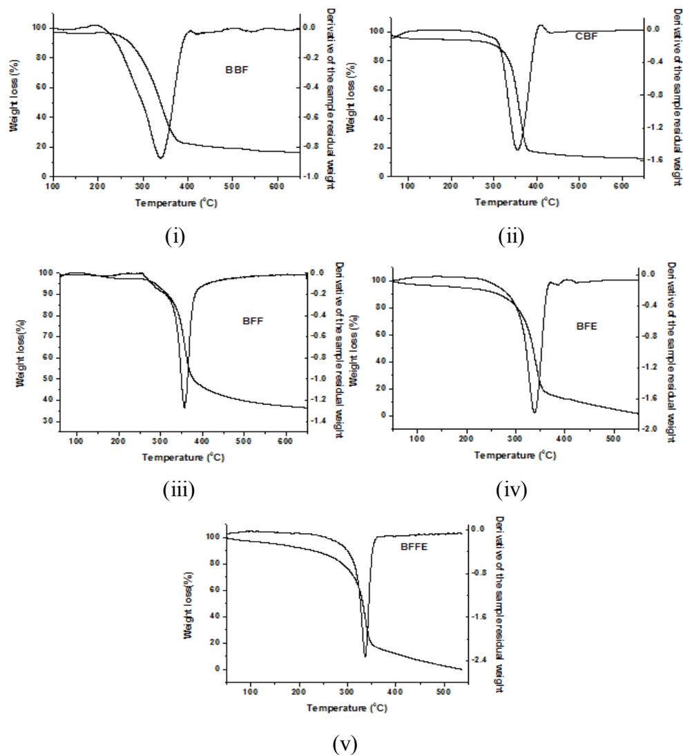
**Figure: 4.23** TG -DTG curves for (i) BBF (ii) CBF (iii) BFF (iv) BFE (v) BFFE
