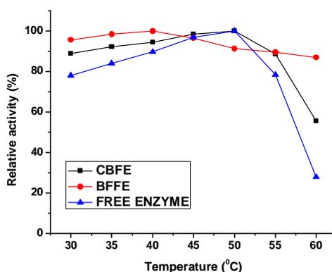
**Figure: 4.33:** Effect of temperature on relative activity of free and immobilized  $\alpha$ -amylase
