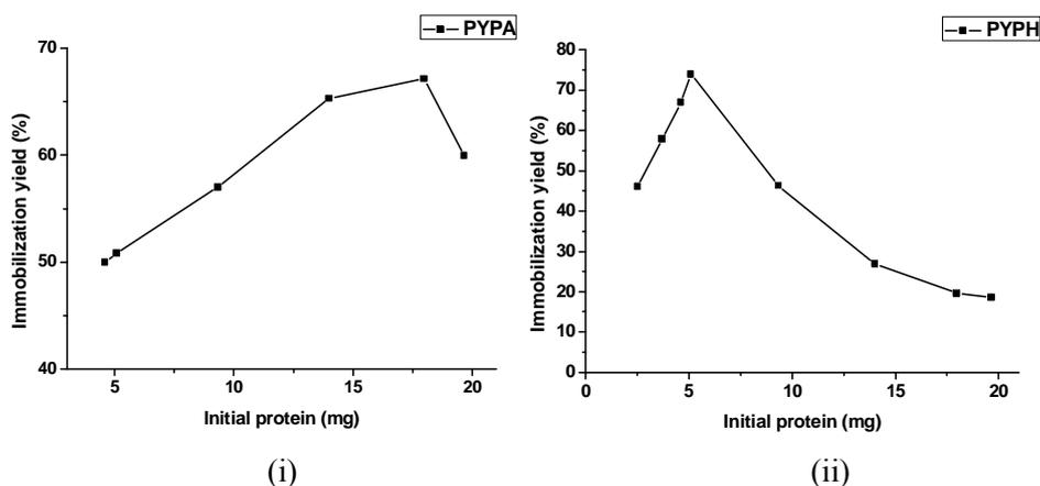
**Figure: 3.56:** Effect of initial protein concentration on the immobilization yield of protein bound on copolymers (i) PYPA (ii) PYPH
