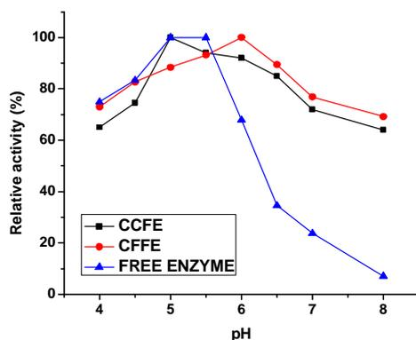
**Figure: 4.13** Effect of pH on the relative activity of free and immobilized  $\alpha$ -amylase
