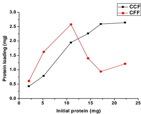
**Figure: 4.10:** Effect of initial protein concentration on the protein loading
