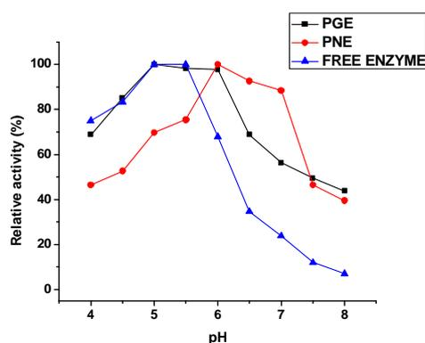
**Figure: 3.43:** Effect of pH on the activity of free and immobilized  $\alpha$ -amylase
