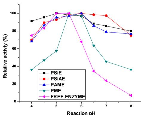
**Figure: 3.73:** Effect of pH on the relative activity of immobilized  $\alpha$ - amylase
