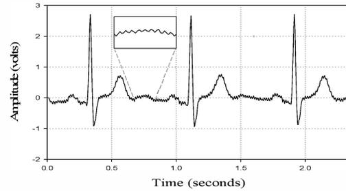
Fig 4. ECG Corrupted with 60Hz PLI
