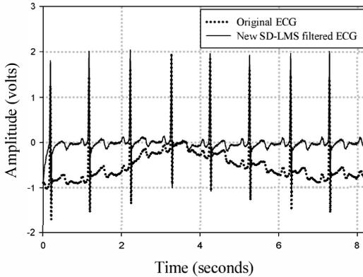
Fig. 2. Results obtained for the removal of BW with the new SD-LMS
