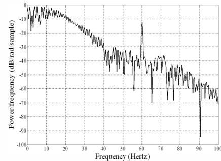
Fig. 6. Peridogram PSD of ECG with 60 Hz interference
