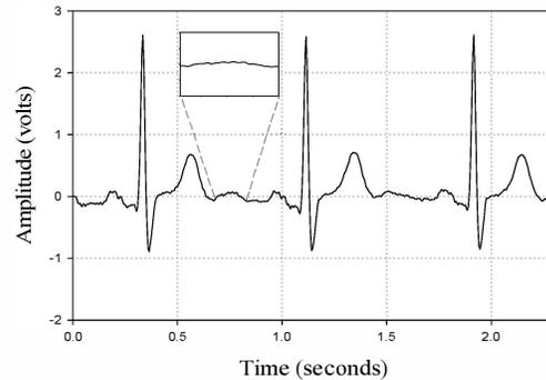
Fig. 5. ECG filtered for PLI with the new SD-LMS filter
