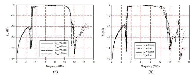
**Figure 6.** Parametric analysis. (a) Dependence of upper cut off frequency on coupled arm length  $L_a$ . (b) Variation of lower cut off frequency with inductive stub length  $L_{stub}$ .
