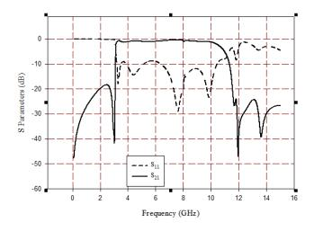
Figure 2. Simulated S parameters.
