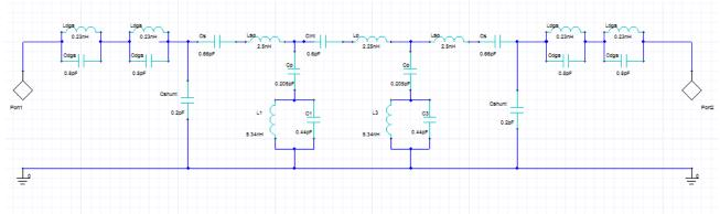
Figure 5. LC equivalent circuit of the filter.
