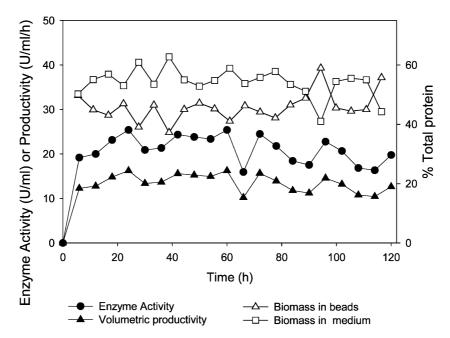
Fig. 2. PBR performance and variation of biomass concentration upon continuous production of L-glutaminase by Ca-alginate immobilized cells.
