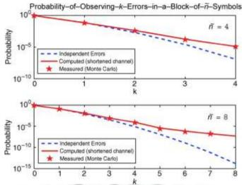
Figure. 7. Error statistics for blocks of 4 and 8 symbols for the channel of Fig. 3(a) with a threshold bias of 36 mV. The results computed analytically based on a shortened channel with l=16 by considering all  $2^{n+l-1}$  symbol patterns match closely the Monte Carlo measurements  $(2.5 \times 10^7 \text{ symbol blocks})$  for the actual (unshortened) channel. The corresponding result based on the independent-errors assumption is also included.
