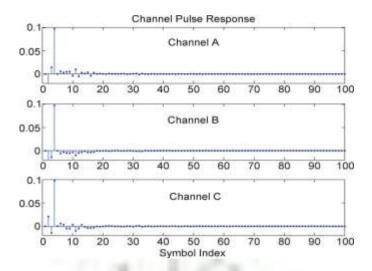
Figure. 3. Equalized pulse response of the standard 802.3ap B32 [10] channel operating at 10 Gb/s. Channel A: Actual channel. Channel B: All-positive signature. Channel C: Randomly generated signature.
