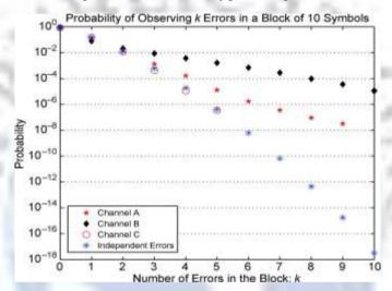
Figure. 4. Joint error statistics for the channels of Fig. 3. Margining by 36 mV increases the error rate to  $1.78 \times 10^{-2}$ , rendering the higher-order error events observable through Monte Carlo simulation ( $2.5 \times 10^{-7}$  symbol blocks). The figure illustrates the extent to which channel signature affects the joint error behavior of the system.
