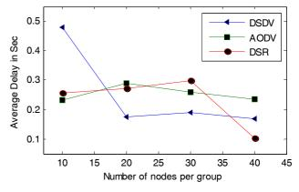
Fig. 5. Delay variation against the number of nodes in RPGM model
