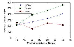
Fig. 4. Delay variation against the number of nodes in Freeway model
