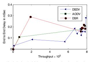
Fig. 3. End-to-End delay variations against throughput in Manhattan mobility model
