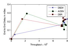
Fig. 1. End-to-End delay variations against throughput in Freeway mobility model
