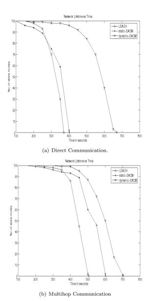
Figure 6. Network lifetime comparison of LEACH, static-EACM and dynamic-EACM.
