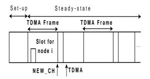
Figure 1. Network operation of static-EACM
