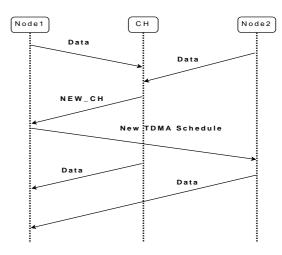
Figure 2. Network operation of static-EACM
