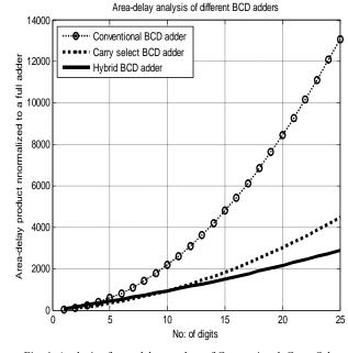
Fig. 4: Analysis of area-delay product of Conventional, Carry Select and Hybrid BCD Adders
