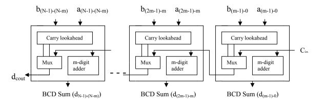
Fig 2. Hybrid N-digit Decimal Adder
