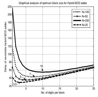
Fig. 10: Graphical analysis of optimum block size of Hybrid reversible BCD adder for different input lengths
