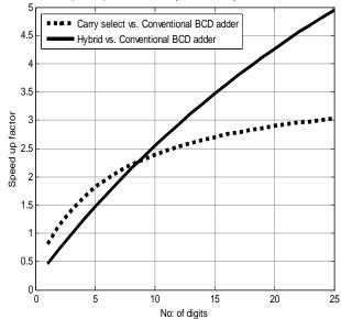
Fig. 5. Speed up factor for Carry select and Hybrid BCD adders vs. conventional BCD adder
