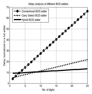
Fig. 3: Delay analysis of Conventional, Carry Select and Hybrid BCD Adders
