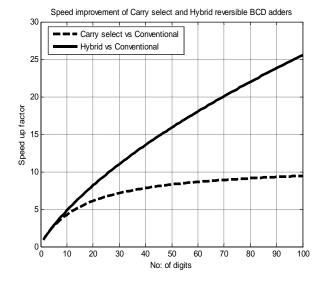
Fig. 12: Speed up factor for VLSI reversible implementations of fast BCD adders vs. Conventional BCD adder
