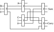
Fig. 7: Full adder using Fredkin Gates
