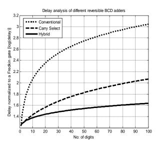
Fig. 11: Delay analysis of VLSI implementations of BCD adders
