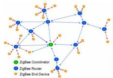
Figure 1-Typical ZigBee WSN – Mesh Architecture
