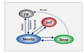
Figure 3 - Sensor Node State Transition
