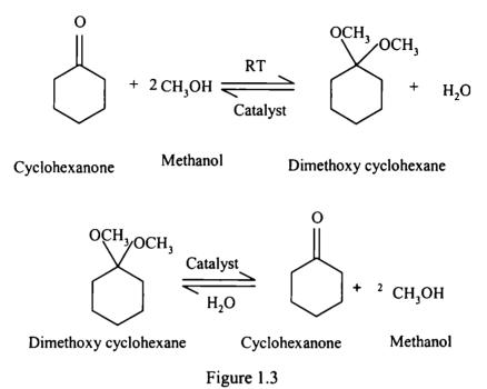
Reaction scheme for acetalization and de-acetalization reaction
