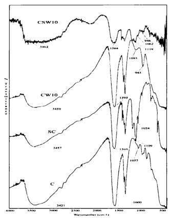
Figure 3.10 FTIR spectra of pure ceria, sulphated ceria, tungsten doped ceria and its sulphated analogues
