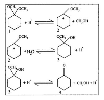
Scheme 2. Mechanism of the hydrolysis of dimethoxy cyclohexane.
