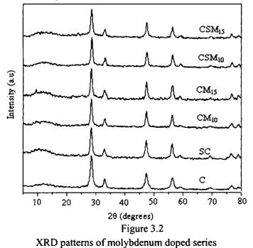
The power X-ray diffraction patterns of the molybdenum loaded catalysts are shown in Figure 3.2. Here also the fluorite structure (space group Fm3m) of ceria is observed in all cases. No characteristic peak of crystalline MoO<sub>3</sub> is observed.
