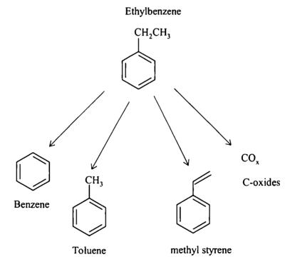
Figure 1.4 Reaction scheme for oxidative dehydrogenation of ethylbenzene
