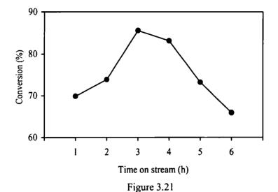
Effect of reaction time on cyclohexanol decomposition reaction Catalyst-0.5 g  $CM_{10}$ , flowrate-4 mL/h, temperature - 300 °C
