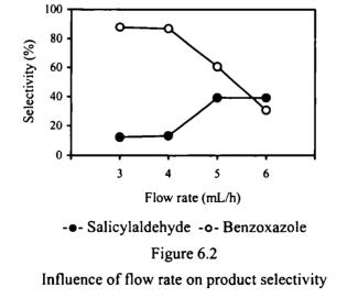
Catalyst-0.5 g CM<sub>15</sub>, reaction temperature-200 °C, time on stream -2 h
