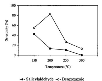
Figure 6.1 Influence of temperature on product selectivity Catalyst-0.5 g CM<sub>15</sub>, flow rate-4 mL/h, time on stream -2 h
