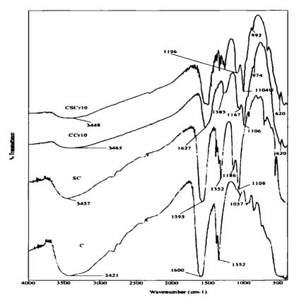
Figure 3.12 FTIR spectra of chromium incorporated systems
