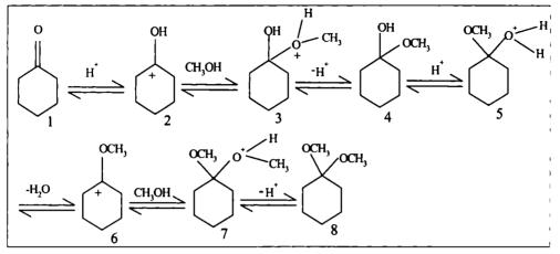
Scheme 1 Mechanism of acetalization of cyclohexanone using methanol
