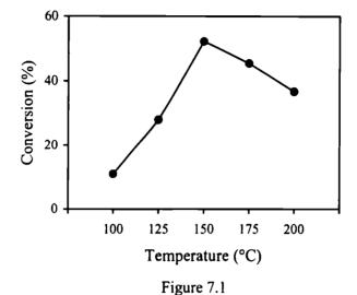
The effect of temperature on conversion in MTBE synthesis. Catalyst  $-0.5 \text{ g CSW}_{15}$ , molar ratio of methanol to tert-butanol-10:1. TOS- 2 h, flow rate-4 mL/h
