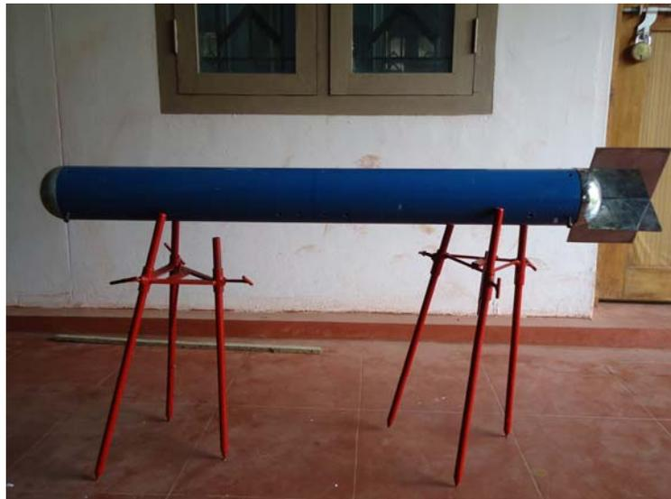
Figure 8.10 Finished assembly of the towed body
