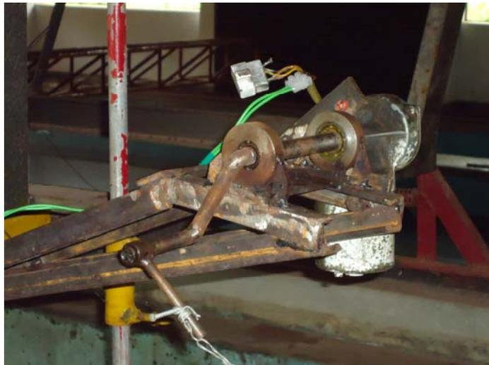
Figure 8.8 Sinusoidal wave motion mechanism
