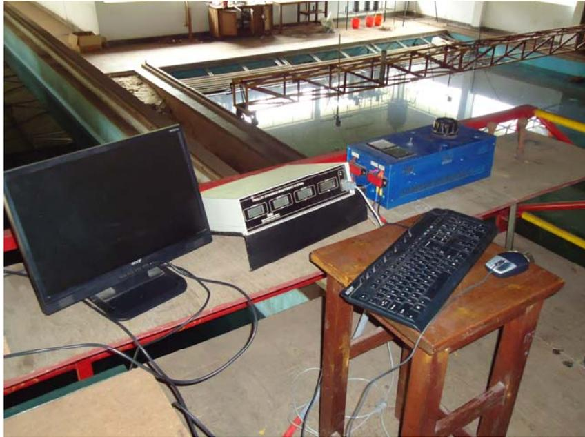
Figure 8.11 Carriage speed control
