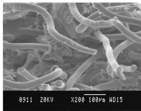
**Figure 3.54 SEM photographs of fracture surface of latex masterbatch composite with HRH**
