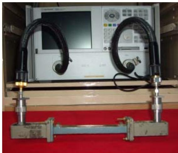
**Figure 6.1 Setup for the measurement of microwave properties**
