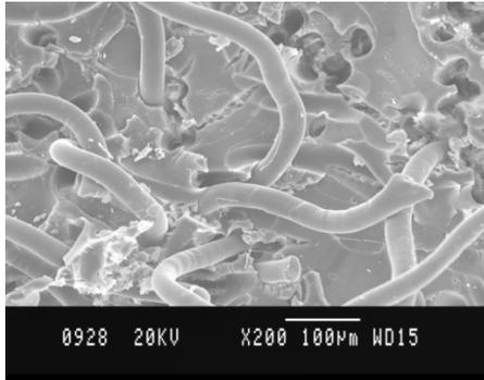
**Figure 3.51 SEM photograph of fracture surface of dry rubber composite**
