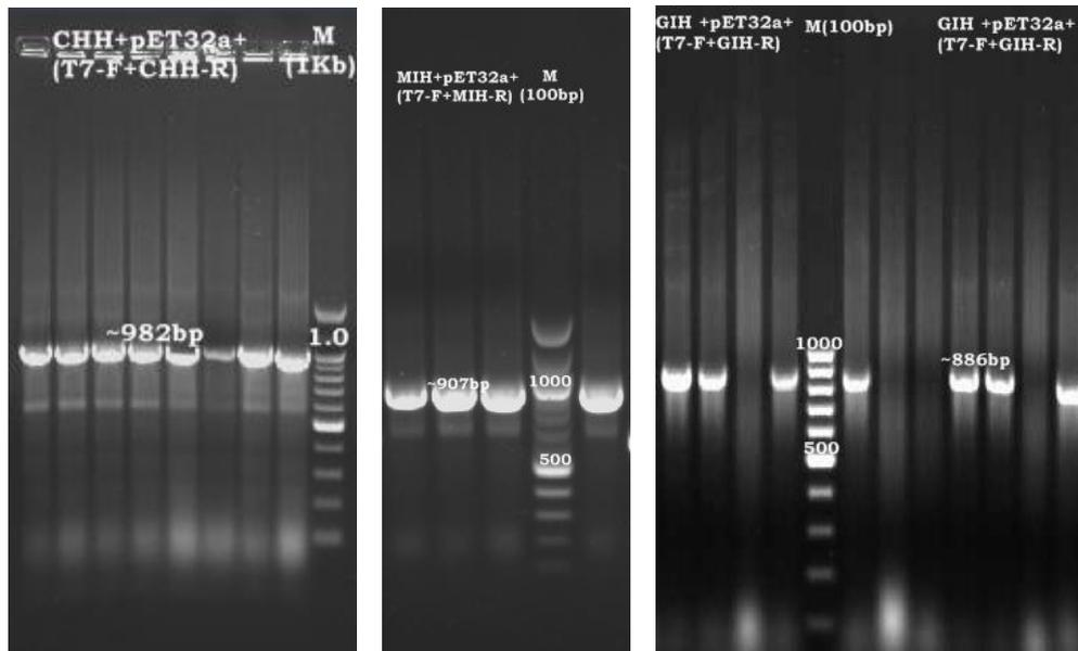
Fig. 8, 9, 10. Insert orientation PCR using forward vector primer and gene specific reverse CHH1 (982 bp), MIH1 (907 bp) and GIH (886 bp).
