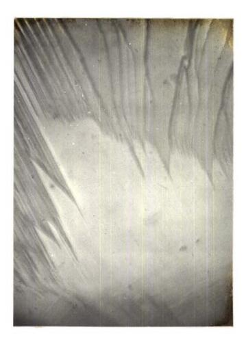
Fig.8.10 A stepped tilt boundary observed on the cleavage surface. (x100)
