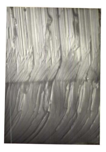
Fig.8.2 A hackle pattern observed on the cleavage face of DAHC. (x600)
