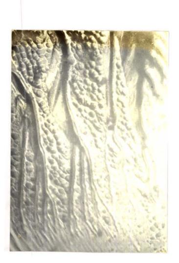
Fig.8.6 An etched cleavage surface containing river patterns. (x200)
