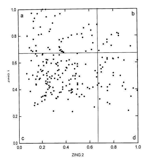
Fig. 7.8 Plot of Zing1 vs. Zing2 for particles from 7 samples for which quantitative measurements were made. For all plots, Zing1=b/a, Zing2=c/b, (a=maximum dimension, b=intermediate dimension and c=minimum dimension). Field a-represents tabular shape, b-represents the equant shape, c-represents the bladed shape and d-represents the prolate shape.
