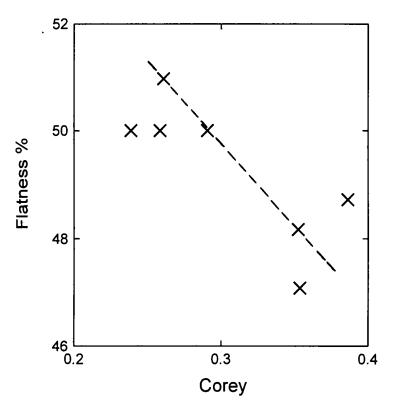
Fig. 7.16b A plot of the average flatness vs the average Corey shape factor for seven samples for which quantitative measurements were made
