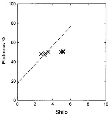
Fig. 7.12b A plot of the average flatness vs the average Shilo factors for 7 samples for which quantitative measurements were made. The curve indicates that the estimated flatness alues are likely to err towards a lower flatness.
