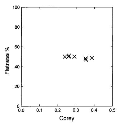
Fig. 7.15b A plot of the average flatness vs the average Corey shape factor for 7 samples for which quantitative measurements were made.
