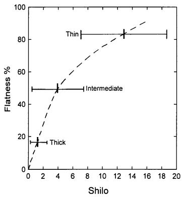
Fig. 7.12a A plot of flatness vs Shilo shape factor for individual particles from samples for which quantitative measurements were made. The horizontal bar represents1 sigma on either side of mean.
