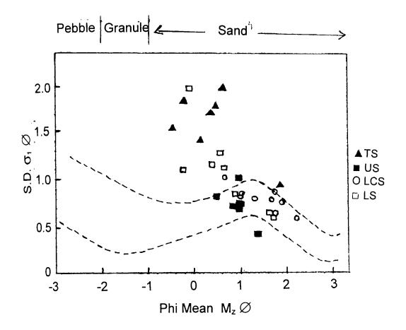
Fig. 3.4 Scatter plot of selected Folk and Ward statistical parameters. Sinusoidal field represent samples having unimodal distribution (after Andrews and Van der Lingen, 1969). Symbol legends as in Fig. 3.5.
