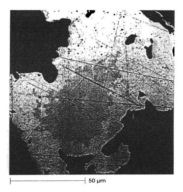
Fig. 7.17 Grains showing rim and core relationship suggesting leaching processes. Note rims are more lighter and show high purity Au while the core is darker and impure. (Grain 2 : Punna puzha).
