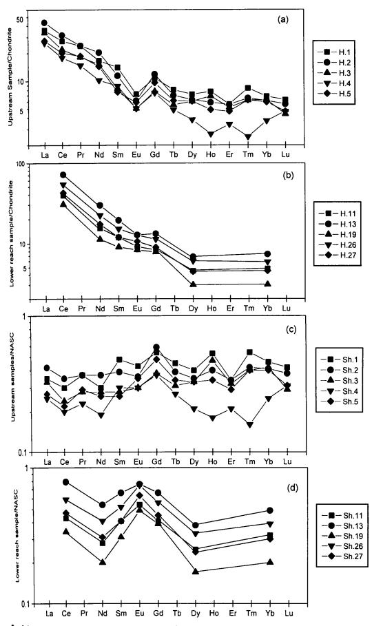
59.6.2 Chondrite-normalised REE pattern of Chaliyar river sediments (a) Upstream (b) Lower reaches Shale-normalised REE pattern of Chaliyar river sediments (c) Upstream (d) Lower reaches
