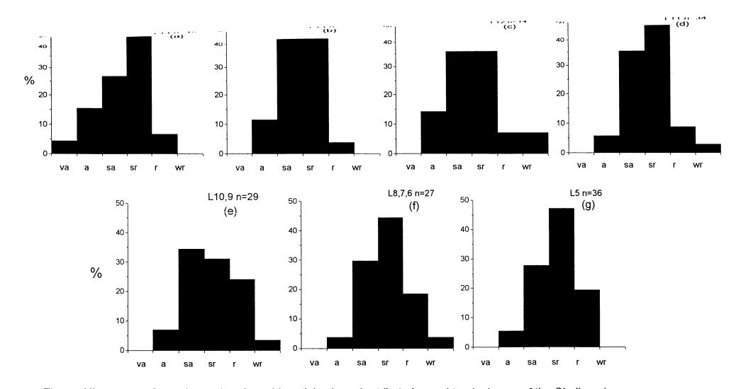
Fig. 7.5 Histograms of roundness data for gold particles in major tributaries and trunk placers of the Chaliyar river (va = very angular; a = angular; sa = sub-angular; sr = sub-rounded; r = rounded; wr = well rounded) (n = number of gold grains)
