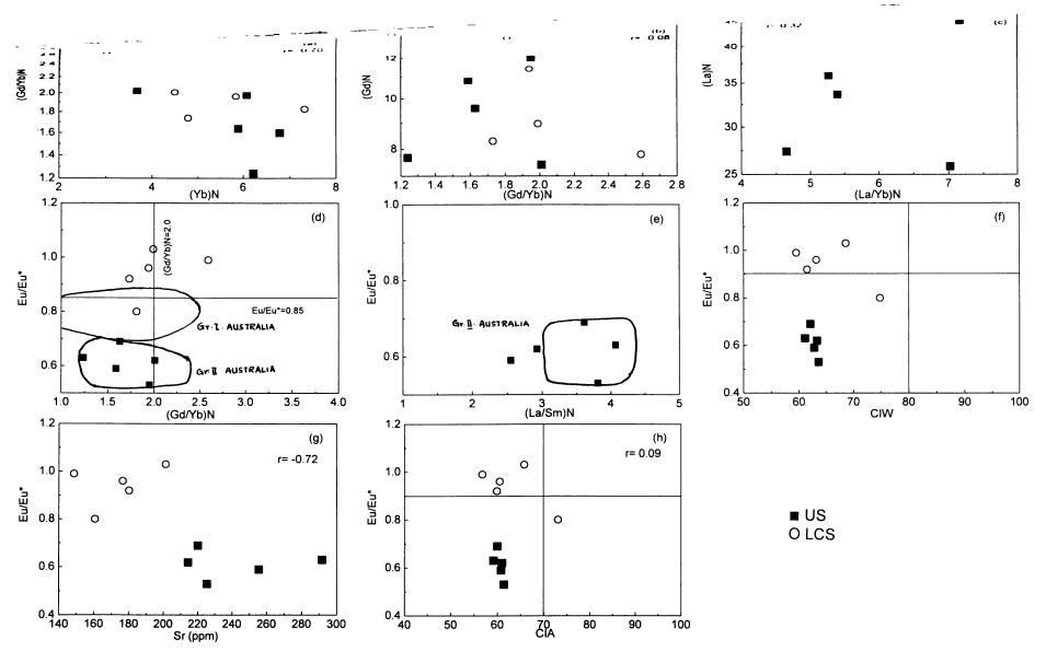
Fig.6.4 Plot of : (a) (Gd/Yb)N vs (Yb)N (Zircon addition); (b) (Gd)N vs (Gd/Yb)N (Monazite addition; (c) (La)N vs (La/Yb)N (Allanite addition); (d) Eu/Eu\* vs (Gd/Yb)N; (e) Eu/Eu\* vs (La/Sm)N; (f) Eu/Eu\* vs CIW; (g) Eu/Eu\* vs Sr (ppm); (h) Eu/Eu\* vs CIA correlations for Chaliyar river sediments
