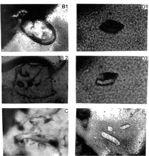
Zircon (B1, B2), Sillimanite (C), Sphene (D1, D2) and Apatite (E) inclusions within Quartz.A, B 1, C, D 2 and E under crossed nicols; B2 and D1 under open nicols. (B1, D1, D2  $\notin$  E: X 250; B2:50; C: X 125)
