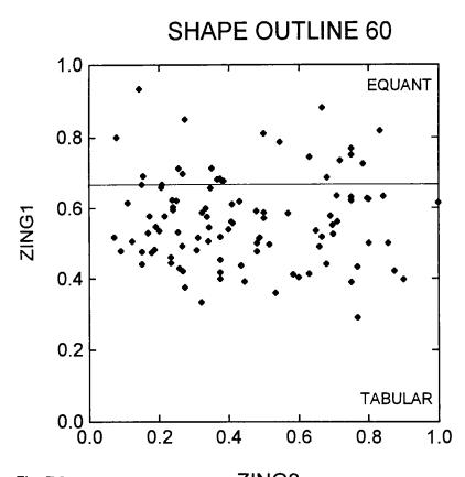
Fig. 7.7cZING2Plot of Zing1 vs Zing2 for particles with a 60 or Complex Outline.Complex shapes should fall close to the line
