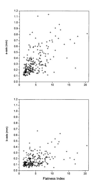
Fig. 7.10 Cailleux flatness index [(a+b)/2c] vs a-axis and b-axis length for all gold particles in Chaliyar river
