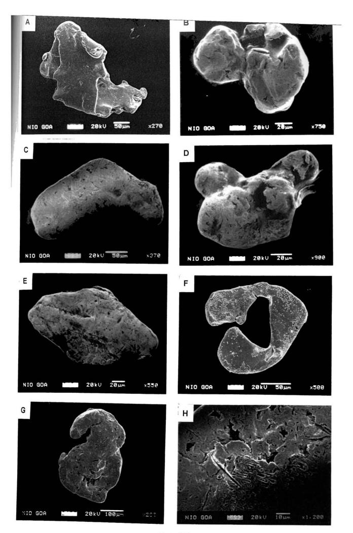
A : Flattened main stem grain showing surface striations (44/L5); note small petal of secondary gold formed in a pit.
