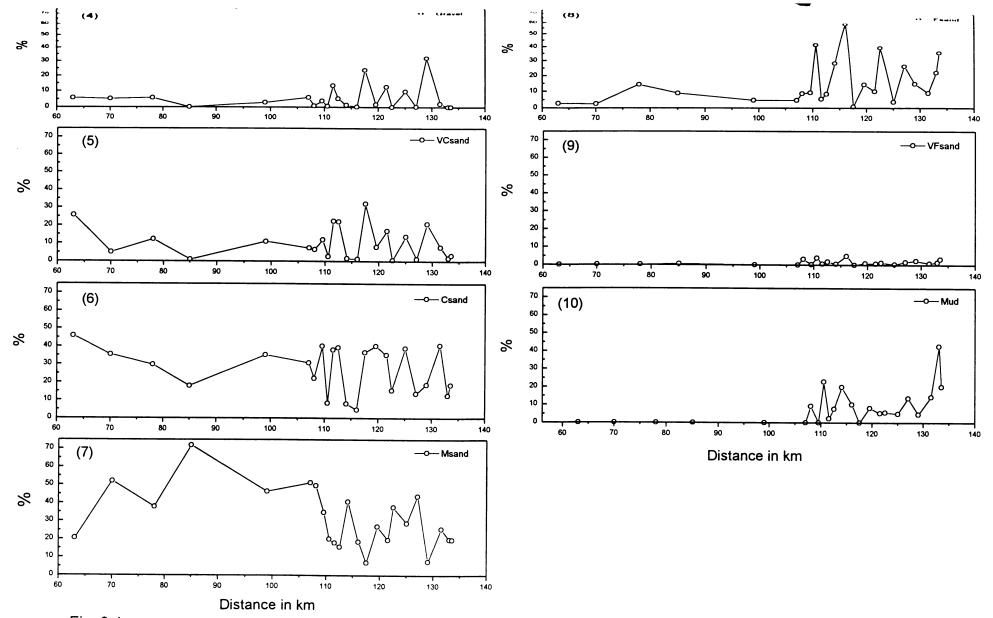
Fig. 3.1a Variations of grain size fractions with distance in the sediments of the Chaliyar river main stem.
