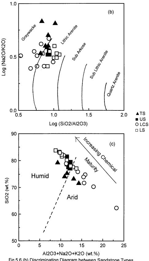
Fig.5.6 (b) Discriminating Diagram between Sandstone Types (after Pettijohn et al., 1973). (c) SiO2 and Al2O3+K2O+Na2O Binary Plot for Sandstones (after Suttner and Dutta, 1986)
