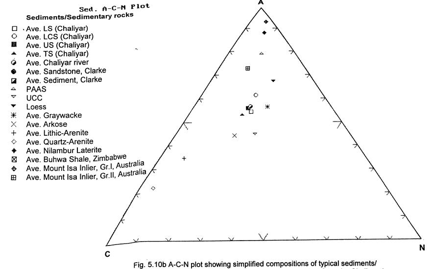
Fig. 5.10b A-C-N plot showing simplified compositions of typical sediments/ sedimentary rock types plotted along with sediment suites from the Chaliyar river.
