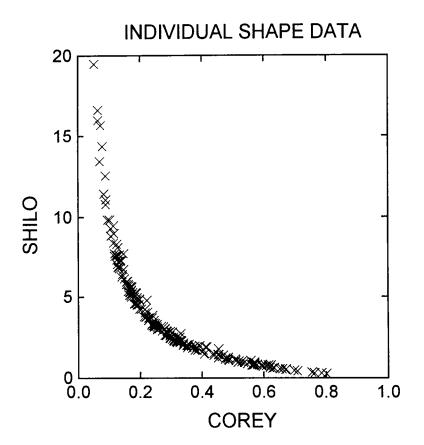
Fig. 7.13 A plot of Shilo vs Corey Shape Factor for individual particles from samples for which quantitative measurements were made
