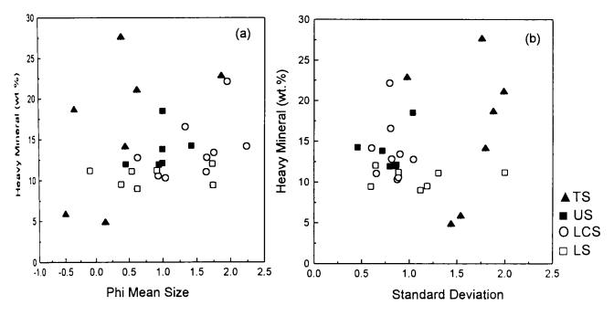
Fig.4.5 Bivariet plot showing relationship between heavy mineral percentage and textural parameters (phi mean size and standard deviation)
