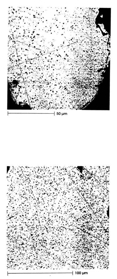
Fig. 7.19 & Fig. 7.20 Polished sections showing differences in the pore densities (Fig. 7.19 Grain 1 : Chali puzha) (Fig. 7.20 Grain 1 : Nilambur, main stem sample)
