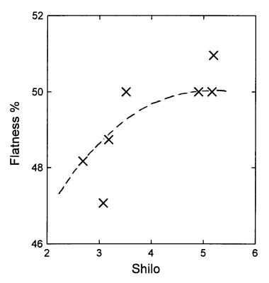
Fig. 7.16a A plot of the average flatness vs the average Shilo shape factor for seven samples for which quantitative measurements were made. The data shows a curvelinear nature.
