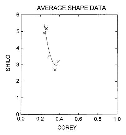
Fig. 7.14 A plot of the average Shilo vs average Corey Factor from 7 samples for which quantitative measurements were made
