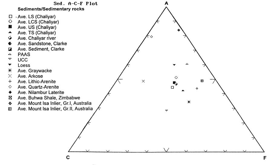
Fig. 5.11b A-C-F plot showing simplified compositions of typical sediments/ sedimentary rock types plotted along with sediment suites from the Chaliyar river.
