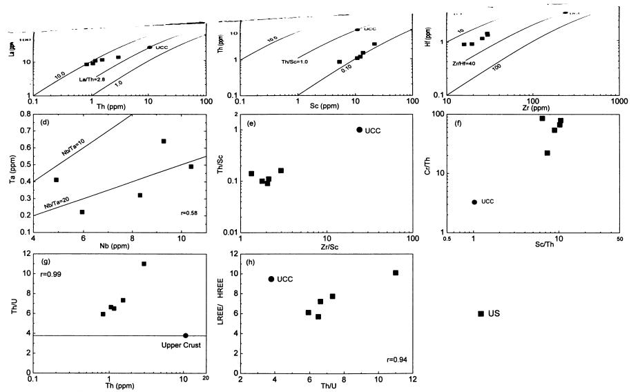
Fig.6.5 Plot of (a) La (ppm) vs Th (ppm); (b) Th (ppm) vs Sc (ppm); (c) Zr (ppm) vs Hf (ppm); (d) Nb (ppm) vs Ta (ppm); (e) Th/Sc vs Zr/Sc; (f) Cr/Th vs Sc/T Weathering trends diagrams (g) Th/U vs Th (ppm); (h) Th/U vs LREE/ HREE for Chaliyar river sediments. UCC = Upper Continental Crust
