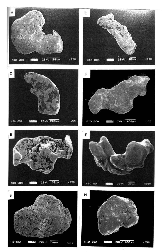
**A**, **B** : Flattened and irregular particles from main stem showing protuberances formed possibly due to hammering; (68/L8,7,6), (69/L8,7,6).
