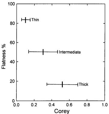
Fig. 7.15a A plot of the flatness vs Corey shape factor for individual particles from samples for which quantitative measurements were made. The horizontal bar represents 1 sigma on either side of the mean.
