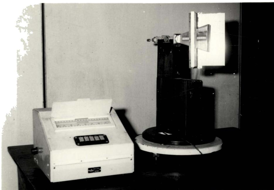
Fig.3.2(a) The turn-table used for plotting the radiation patterns manually.
