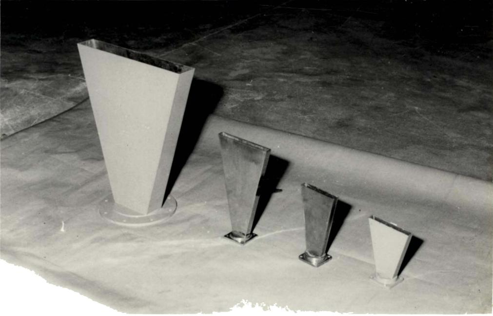
Fig.3.1(iii)(a) The sectoral horns used in this study.
