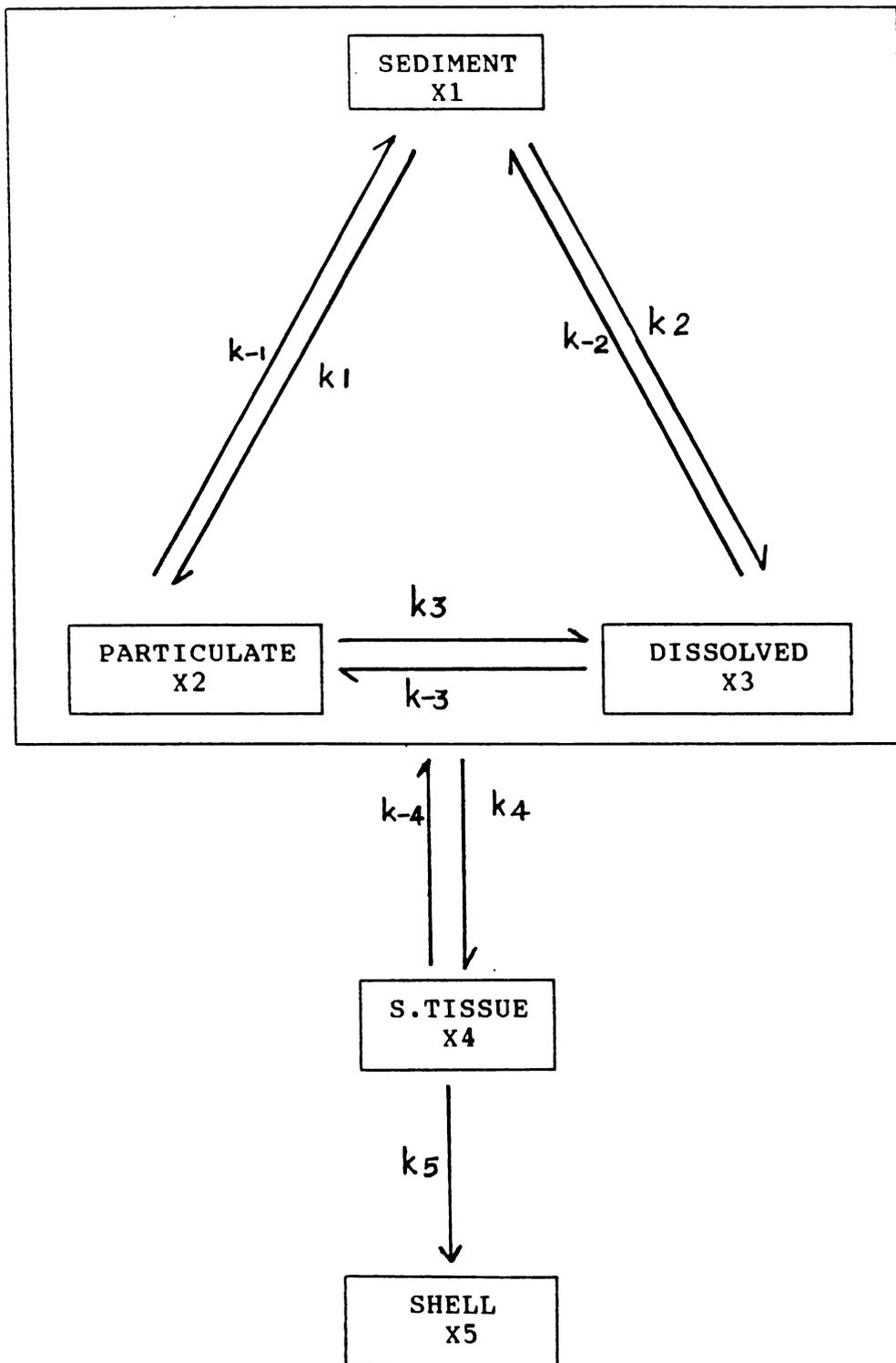
**Fig.36 Trace metal partitioning in an estuarine system**
