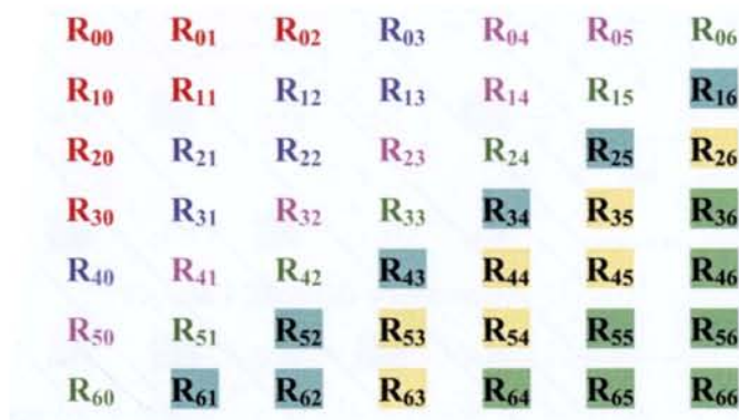
Figure 2.24: Register array for storing output of BCD-digit multiplication
