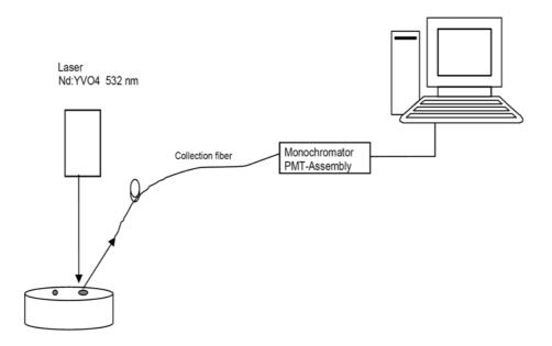
Figure: 7.2. Experimental setup to study the growth kinetics of bacterial colony by using Laser Induced Fluorescence technique
