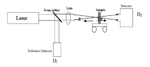
Figure 2.2. Schematic representation of the experimental set up for Z-scan technique.
