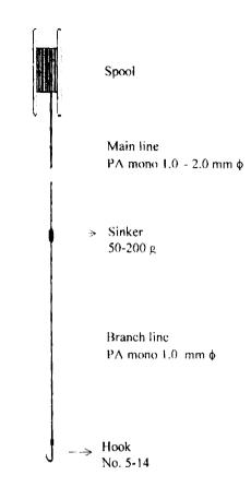
Fig. 135. Eruchoonda with single hook
