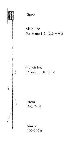
Fig. 136. Eruchoonda with multiple hooks
