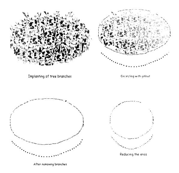
Fig. 155. Operation of FADs in rivers of Central Kerala
