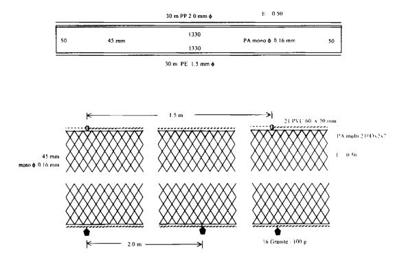
Fig. 40. Experimental gillnet for mesh selectivity studies with 45 mm meshes
