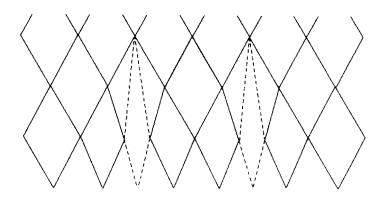
Fig. 94. Fly mesh using in the cast net fabrication
