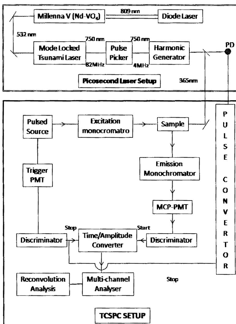
**Figure 4.** Diagram representing the TCSPC and Picosecond Laser setup
