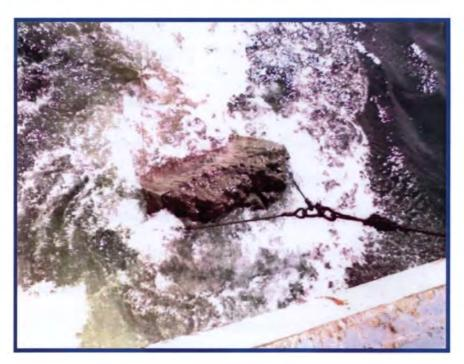
Fig.6.1. Operation of rectangular dredge for collecting epifauna
