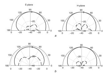
Fig. 5 E-plane and H-plane radiation characteristics of proposed antenna a At port 1 b At port 2
