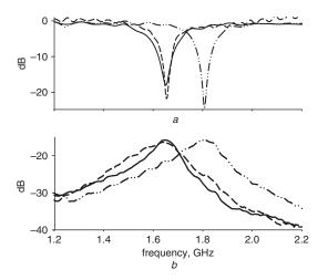
Fig. 4 Measured reflection and transmission characteristics of antenna a Reflection characteristics
