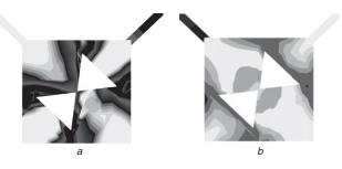
**Fig. 2** *Current path on patch a* Port 1 excited *b* Port 2 excited
