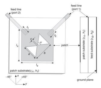
Fig. 1 Geometry of proposed antenna
