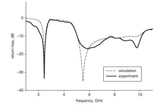
Fig. 2 Simulated and measured return loss characteristics of antenna structure
