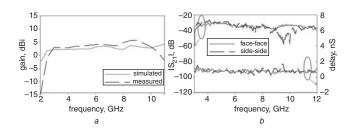
Fig. 5 Measured peak gain and group delay and  $|S_{21}|$  of antenna a Peak gain
