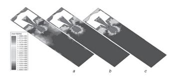
Fig. 3 Surface current distribution on antenna integrated with PCB of USB dongle at 3.35, 6.5, 10 GHz
