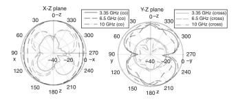
Fig. 4 Measured radiation patterns of antenna
