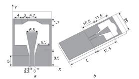
Fig. 1 Proposed antenna a Geometry b Integrated with WUSB dongle PCB
