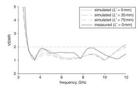
Fig. 2 VSWR plot of antenna for different ground lengths
