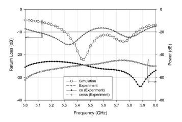
**Figure 3** Measured return loss, co and cross powers with L = 36 mm,  $L_1 = 23$  mm,  $L_2 = 23$  mm, and  $L_3 = 3$  mm,  $\varepsilon_r = 4.4$  mm, h = 1.6 mm, and Wt = 3 mm
