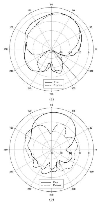
**Figure 4** (a) Measured radiation patterns of the antenna at f = 5.3 GHz. (b) Measured radiation patterns of the antenna at f = 5.8 GHz
