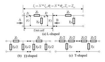
**Figure 1** Three types of general periodical circuit models with L-shaped, II-shaped, and T-shaped
