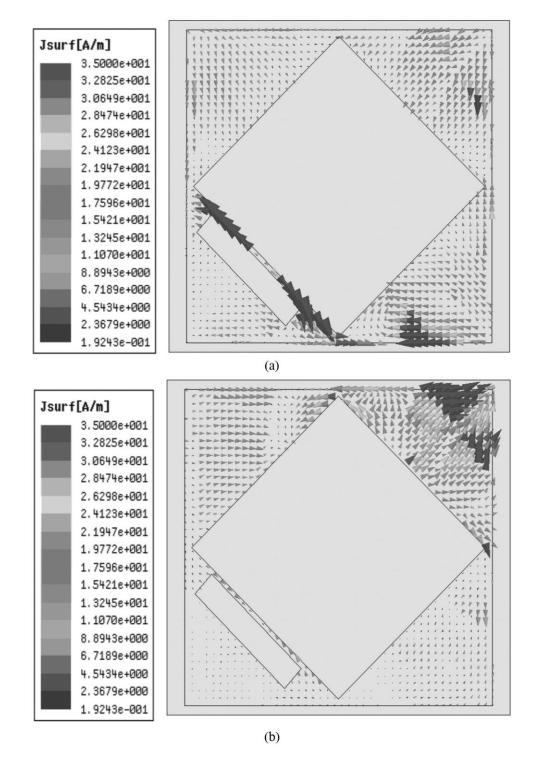
**Figure 5** (A) Simulated surface current distribution of the proposed antenna at f = 5.3 GHz. (b) Simulated surface current distribution of the proposed antenna at 5.8 GHz
