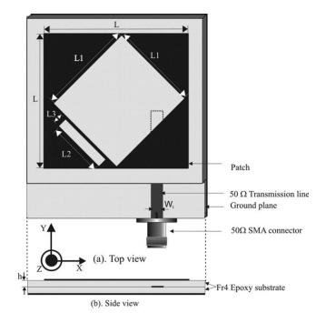
Figure 1 Antenna Geometry
