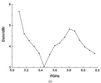
**Figure 6** Peak gain of the proposed dual-band antenna (a) 2.4-GHz band and (b) 5-GHz band
