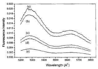
FIGURE 3 Un-normalised fluorescence spectrum for different excitation wavelengths (a) 514 nm, (b) 496 nm, (c) 476 nm, (d) 488 nm, (e) 457 nm
