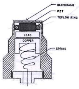
Figure 2s. The PZT transducer.
