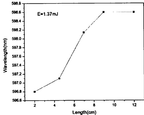
Fig. 8. Variation of laser emission peak with length of the fiber having a diameter of 510  $\mu\text{m}$  at a pump energy of 1.37 mJ/pulse.
