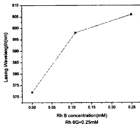
Fig. 4. Tuning of multimode laser emission peak with different dye concentrations. Rh 6G concentration is constant (0.25 mM) in all three samples. Pump energy is 1.37 mJ/pulse.  $L = 7$  cm and  $D = 510 \mu\text{m}$ .
