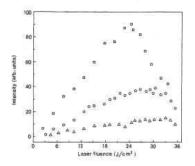
Fig. 5. Change in intensity for second peak with respect to laser fluence at different distances ( $\Box$ ) 5 mm, ( $\bigcirc$ ) 10 mm and ( $\triangle$ ) 15 mm (pressure 0.5 Torr).
