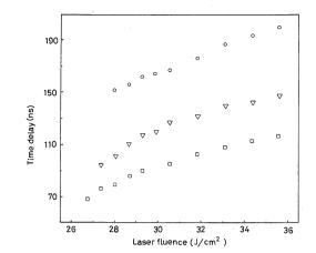
Fig. 2. Variation of time delays with laser fluence for the first peak at distances  $(\Box)$  5 mm,  $(\bigtriangledown)$  10 mm and  $(\bigcirc)$  15 mm (helium pressure 0.5 Torr).
