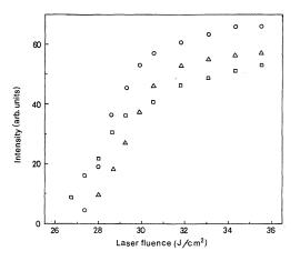
Fig. 4. Change in intensity for first peak with respect to laser fluence at different distances ( $\Box$ ) 5 mm, ( $\bigcirc$ ) 10 mm and ( $\triangle$ ) 15 mm (pressure 0.5 Torr).
