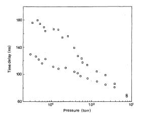
Fig. 6. Dependence of time delays of first peak on ambient helium pressure ( $\bigcirc$ ) 5 mm and ( $\square$ ) 8 mm (laser fluence 30 J/cm<sup>2</sup>).
