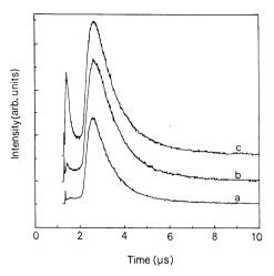
Fig. 1. Intensity variation of spectral emission with time for  $C_2$  observed at 1 cm away from the target for laser fluences (a)  $26.7 \text{ J/cm}^2$  (b)  $27.4 \text{ J/cm}^2$  and (c)  $28 \text{ J/cm}^2$  (helium pressure 0.5 Torr).
