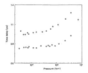
Fig. 7. Dependence of time delays of second peak on ambient helium pressure (○) 5 mm and (□) 8 mm (laser fluence 30 J/cm<sup>2</sup>).
