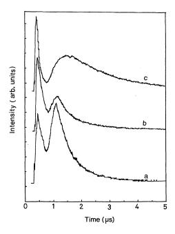
Fig. 8. Intensity variation of spectral emission with time for  $C_2$  observed at 8 mm away from the target at different ambient helium pressures (laser fluence 30 J/cm<sup>2</sup>) (a) 0.05 Torr, (b) 0.8 Torr and (c) 7.5 Torr.
