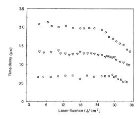
Fig. 3. Variation of time delays with laser fluence for the second peak at distances  $(\Box)$  5 mm,  $(\bigtriangledown)$  10 mm and  $(\bigcirc)$  15 mm (helium pressure 0.5 Torr).
