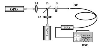
Fig. 1. Schematic diagram of the experimental set up.  $L_1$ ,  $L_2$ , lens; DM, dichoric mirror; S, sample; OF, optic fibre, MPA, monochromator-PMT assembly; DSO, digital storage oscilloscope.
