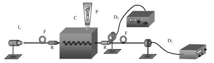
Fig. 1. Schematic diagram of the experimental set-up L: diode laser (633 nm), C: cell containing pH solution, P: pH electrode, F: optical fiber, R: index matching liquid  $D_1$ : detector 1 (Metrologic 45–545),  $D_2$ : detector 2 (Newport 1815-C).
