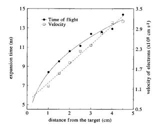
FIG. 3. Variation of the time of flight as well as velocity of electrons with distance from the target.
