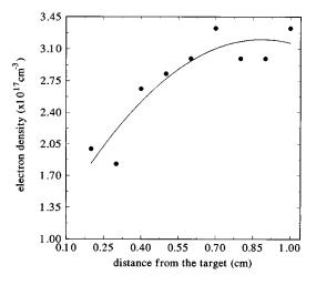
FIG. 5. Variation of prompt electron density as a function of distance from the target at a pressure of 0.27 mbar. The density increases with distance from the target indicating electron generation due to collisions.
