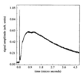
FIG. 1. Temporal profile of the probe signal. The profile shows clear twin peak distribution. The narrow peak appearing early in time represent prompt electrons and the broad peak correspond to the plasma electrons which extends to several microseconds.
