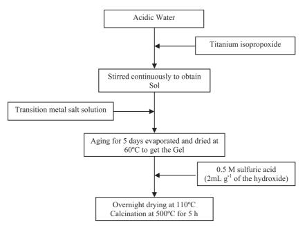
Fig. 1. Preparation process of transition metal loaded sulfated titania powders.
