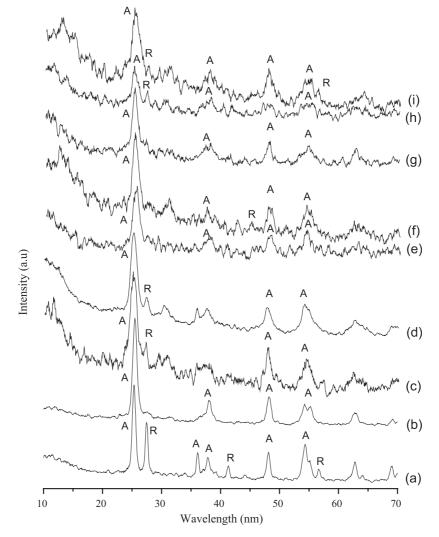
Fig. 2. XRD profiles of T (a), ST (b), STCr3 (c), STMn3 (d), STFe3 (e), STCo3 (f), STNi3 (g), STCu3 (h) and STZn3 (i). A, anatase; R, rutile.
