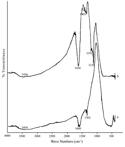
Fig. 3. FTIR spectra of T (a) and ST (b).
