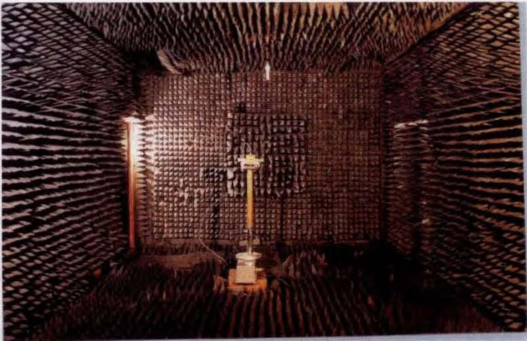
**Figure 3.7** *Microwave Anechoic Chamber where the antenna measurements are made. The antenna positioner interfaced to the network analyzer is also shown*
