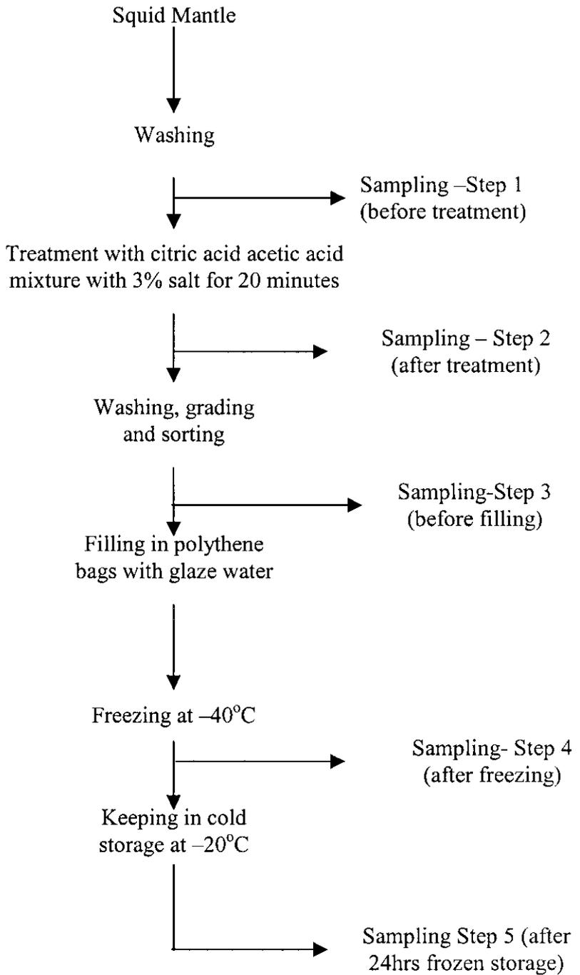
**Figure 4.1. FLOW CHART OF SQUID PROCESSING**
