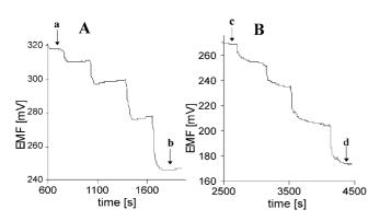
Fig. 3. Dynamic responses of Mn(III)-porphyrin ISE (A) Mn(III)-porphyrin-CPE (B). The analyte concentration was changed from a)  $3.2 \times 10^{-5}$  M to b)  $3.2 \times 10^{-3}$  M (A) and from c)  $3.2 \times 10^{-5}$  M to d)  $2.0 \times 10^{-5}$  M (B).
