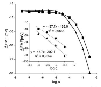
Fig. 2. Potentiometric response toward paracetamol of Mn(III)porphyrin ISE (**n**) and Mn(III)-porphyrin CPE (**a**). The measurements were performed in the presence of  $1.0 \times 10^{-2}$  M phosphate buffer, pH 5.5 (**n**, n = 8; 0.24 < SD < 9.35), (**a**, n = 6; 0.25 < SD <11.92).
