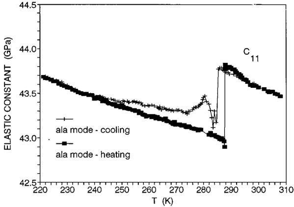
FIG. 2. Temperature variation of elastic constant for the cooling and heating cycle of the *ala* mode in LAS.
