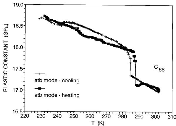
FIG. 3. Temperature variation of elastic constant for the cooling and heating cycle of the *atb* mode in LAS.
