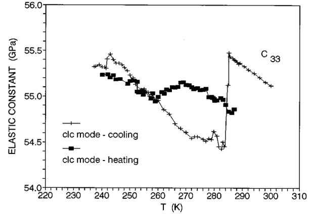
FIG. 4. Temperature variation of elastic constant for the cooling and heating cycle of the *clc* mode in LAS.
