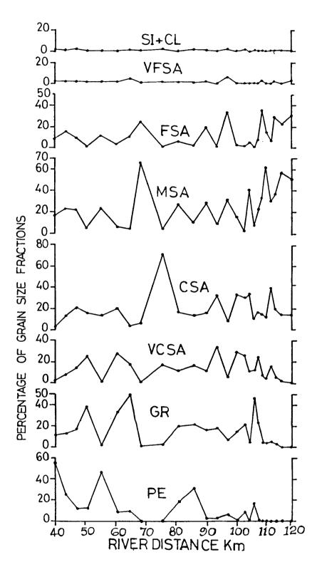
Fig. 6 Downstream variation of grain size fractions through Thodupuzha - Muvattupuzha - Ittupuzha river channels (PE Pebble, GR Granule, VCSA Very coarse sand, CSA Coarse sand, MSA Medium sand, FSA Fine sand, VFSA Veryfine sand and SI+CL Silt + Clay)
