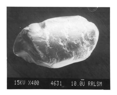
Plate 5a Subrounded estuarine zircon (+120 mesh) showing intense mechanical and chemical surface textures
