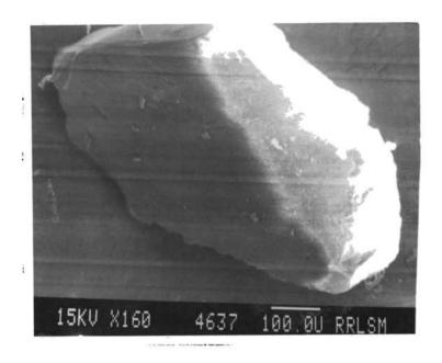
Plate 1a A quartz grain of the Muvattupuzha river (upstream) showing sharp edges and planar surfaces
