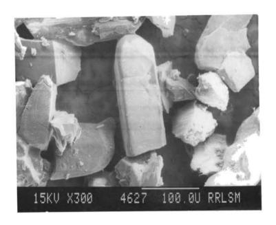
Plate 6a Broken zircon (+230 mesh) in the Muvattupuzha riverine sediments
