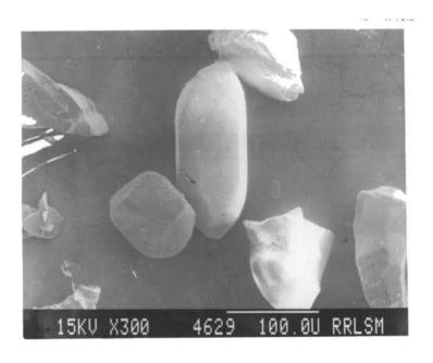
Plate 4b Pyramidally terminated zircon (+230 mesh) with smooth surface. Note the bright ilmenite grain below it
