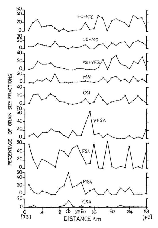
Fig. 7 Variation of grain size fractions in the sediments of Central Vembanad estuary i.e. from Thannirmukham Bund [TB] to Fort Cochin [FC]. (CSA Coarse sand, MSA Medium sand, FSA Fine sand, VFSA Veryfine sand, CSI Coarse silt, MSI Medium silt, FSI+VFSI Fine silt + Veryfine silt, CC+MC Coarse clay + Medium clay); ID Itupuzha distributary, MD Murinjapuzha distributary
