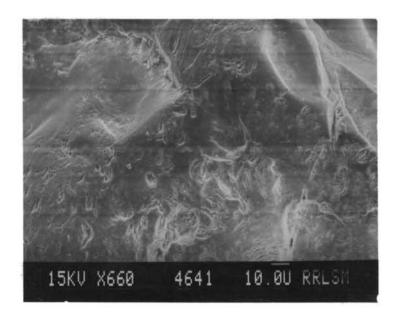
Plate 2b Photomicrograph of estuarine quartz showing pitted surface and diagenetically derived surface textures
