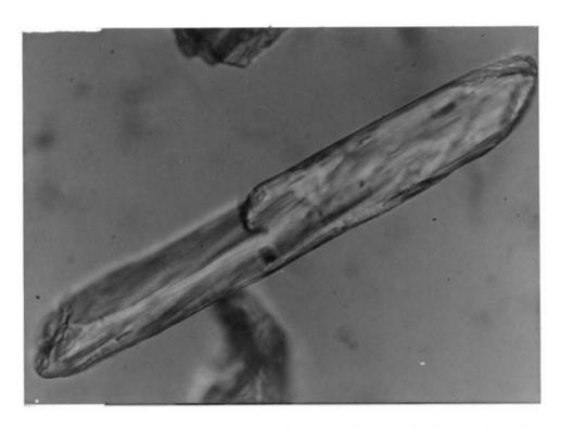
Plate 16a A sillimanite needle with rounded terminations (plane polarised light)
