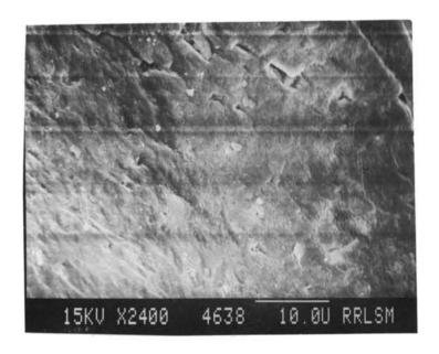
Plate 1b Quartz grain surface (riverine) showing V-pits in initial stages
