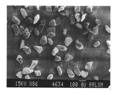
Plate 17b Scanning electron photomicrograph of total heavies in the +230 mesh fraction of Central Vembanad estuarine sediments
