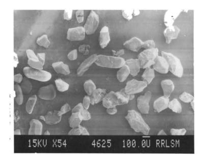
Plate 18a Scanning electron photomicrograph of total heavies in the +120 mesh fraction of Muvattupuzha riverine Sediments
