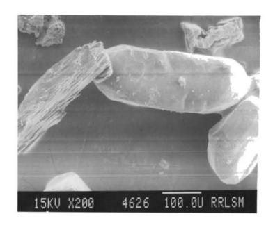
Plate 4a Elongated zircon grain (+120 mesh) with pyramidal terminations. On the left, it is partially overlapped by a book of biotite
