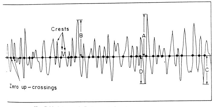
Fig. 3.11 Scheme of Tucker analysis of wave records
