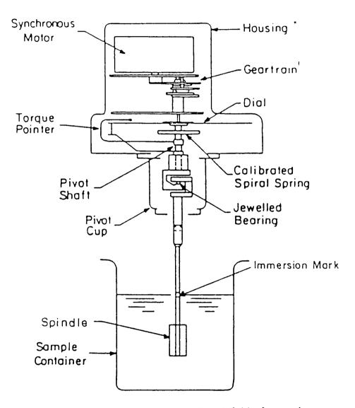
Fig. 3.12 Skeletal structure of Brookfield viscometer
