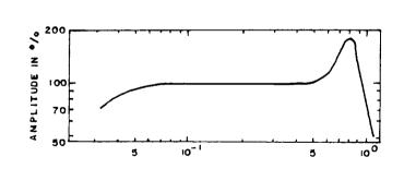
Fig. 3.9 Frequency response of waverider
