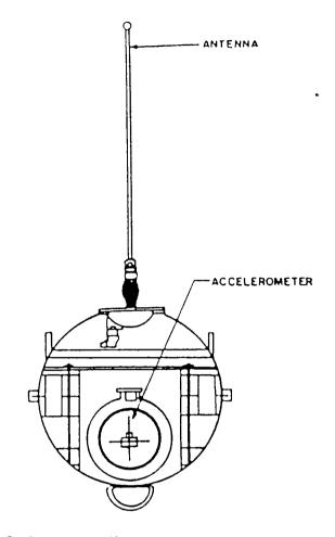
Fig. 3.8 Cross-section of the waverider buoy
