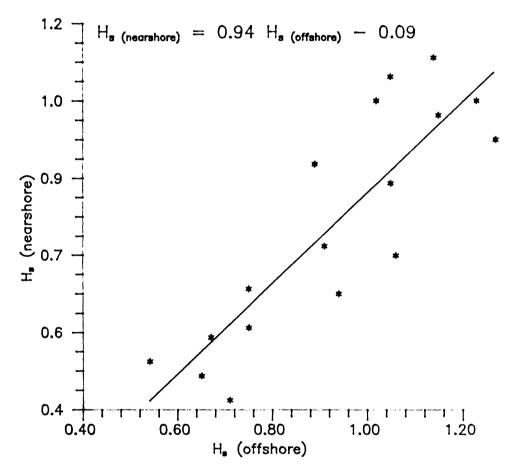
Fig. 4.5 Comparison of synchronous nearshore and offshore significant wave heights in the absence of mudbank
