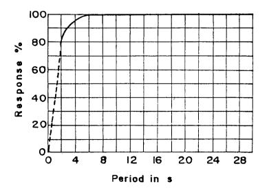
Fig.3.5 Frequency response diagram of wave recorder
