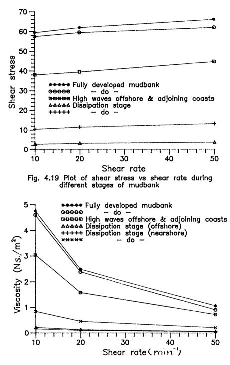
Fig. 4.20 Decrease in viscosity with increase in shear rate
