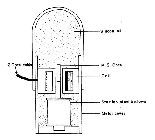
Fig. 3.4 Transducer of wave and tide recorder (Cross section)
