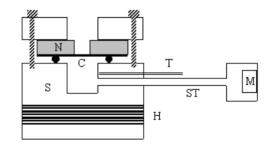
**Figure 2.** Cross-sectional view of the open photoacoustic cell. N is the nylon ring, C the copper foil, T the thermocouple, S the stainless steel body, H the heater coil, ST the stainless steel tube and M the microphone.
