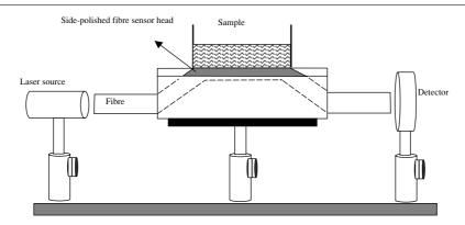
Figure 1. The side-polished fibre optic sensor for the detection of traces of adulterant oils in coconut oil.
