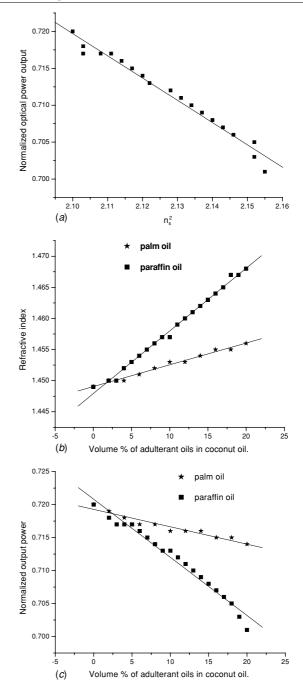
**Figure 2.** (*a*) Variation of the normalized output power *P* with  $n_s^2$  of test samples of paraffin oil in coconut oil. (*b*) The refractive index of sample mixtures against the volume percentage of paraffin oil/palm oil in coconut oil. (*c*) Normalized output power against the volume percentage of paraffin oil/palm oil in coconut oil.
