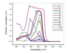
Fig. 2 Net absorption spectra of dye mixture doped PMMA rods along with pure donor emission. 1- [D] only  $(5x10^{-5} \text{ m/l})$ , 2-[A] =4x10<sup>-5</sup>, 3- [A] = 7x10<sup>-5</sup>, 4- [A]= 10<sup>-4</sup>, 5- [A]= 2x 10<sup>-4</sup>, 6- [A] = 4x 10<sup>-4</sup>, 7- [A] = 5x10<sup>-4</sup>, 8 - [A] = 6x10<sup>-4</sup>, 9-[A] = 7x10<sup>-4</sup>, 10-[A] (10<sup>-4</sup> m/l) only, 11- donor emission
