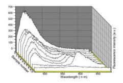
Fig. 3 The recorded fluorescence from dye mixture doped PMMA with 465 nm excitation.
